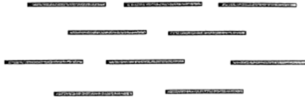
Figure 2. Contour Log Terrace. These barriers are an effective, first-year treatment for hydrophobic soils, low ground cover density, and severely burned areas (graphic courtesy of Natural Resources Conservation Service.)
