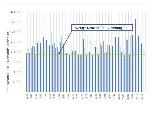
Figure 2. Total Projected Demands for the Decker Creek Power Station and Fayette Power Project
