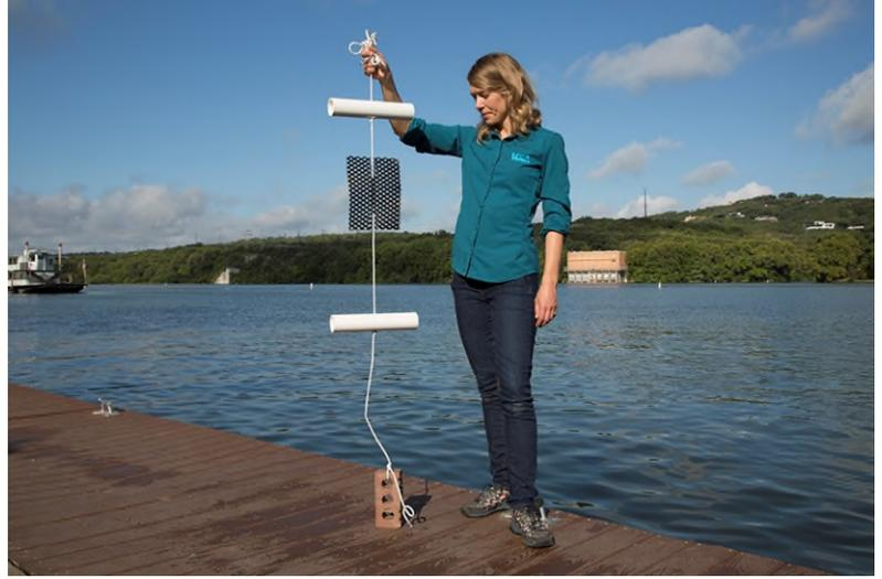
A zebra mussel settlement sampler provides an easy, inexpensive way to monitor for zebra mussels, a small invasive species that attaches to solid surfaces in the water. Samplers can be hung from docks, barges or other structures in the water, and should be about 6-8 feet long, if the water is that deep at the deployment site.
