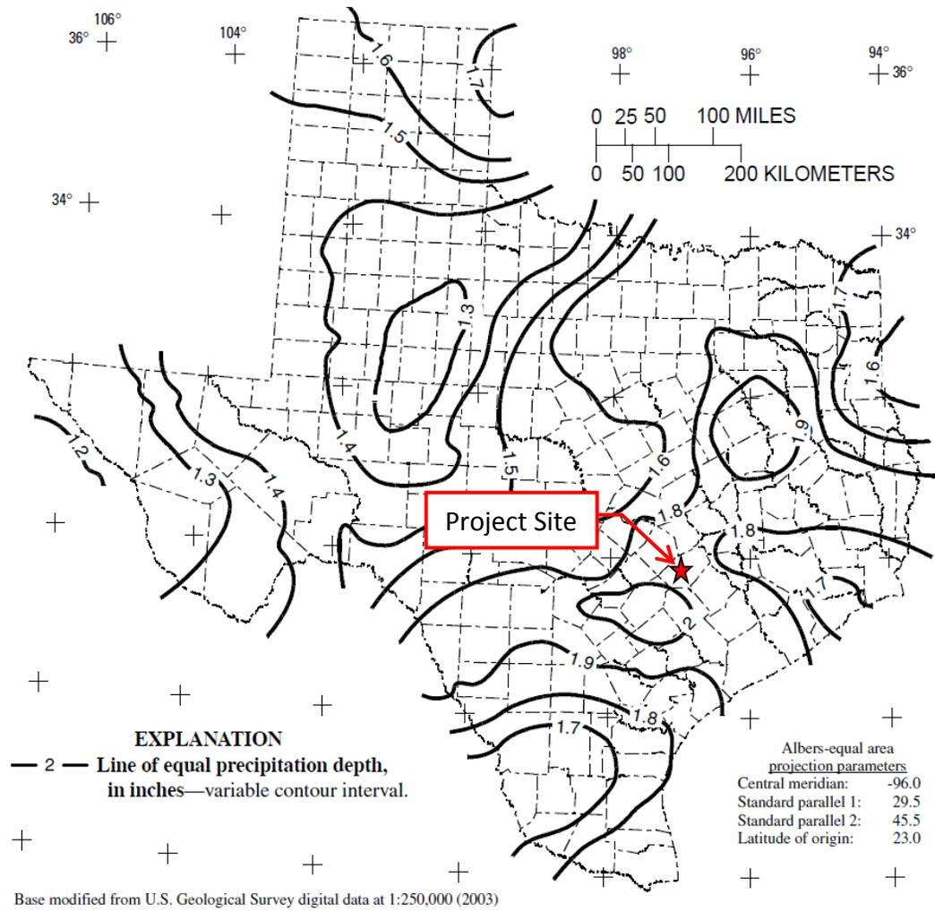
**Figure 6 – Depth of Precipitation for 25-year Storm for 15-minute Duration in Texas (from USGS, 2004)**
